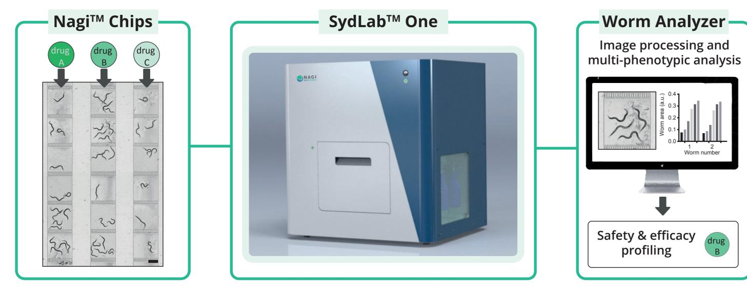
Worms are automatically injected into the microfluidic platform and confined within dedicated chambers of the microfluidic chips. They are then continuously fed with E. coli solution and can be exposed to the test interventions according to a defined treatment plan. Pictures or videos of each micro-chamber **are acquired via time-lapse microscopy** at desired frequency.
